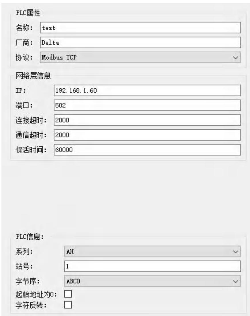
The screenshot shows a configuration window for a PLC. It is divided into three main sections: 'PLC属性' (PLC Properties), '网络层信息' (Network Layer Information), and 'PLC信息' (PLC Information).
