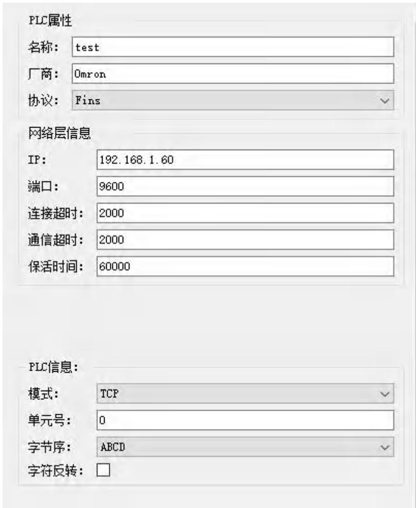
The screenshot shows a configuration window for a PLC. It is divided into three sections: 'PLC属性' (PLC Properties), '网络层信息' (Network Layer Information), and 'PLC信息' (PLC Information).
